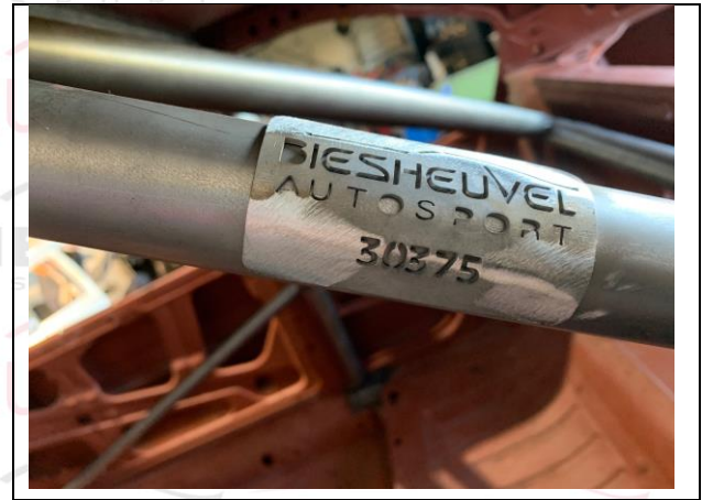
PHOTO 16 DETAILS OF IDENTIFICATION PLATE
