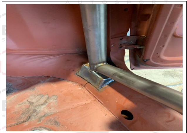
PHOTO 6 FRONT ROLLBAR TO FLOOR ATTACHMENT
