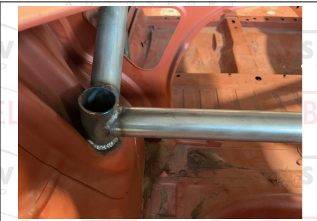
PHOTO 5 REAR BACKSTAY TO BODYSHELL ATTACHMENT
