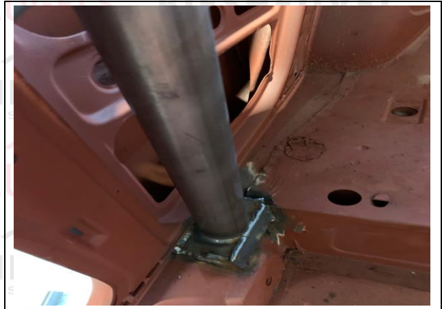
PHOTO 4 MAIN ROLLBAR TO FLOOR ATTACHMENT
